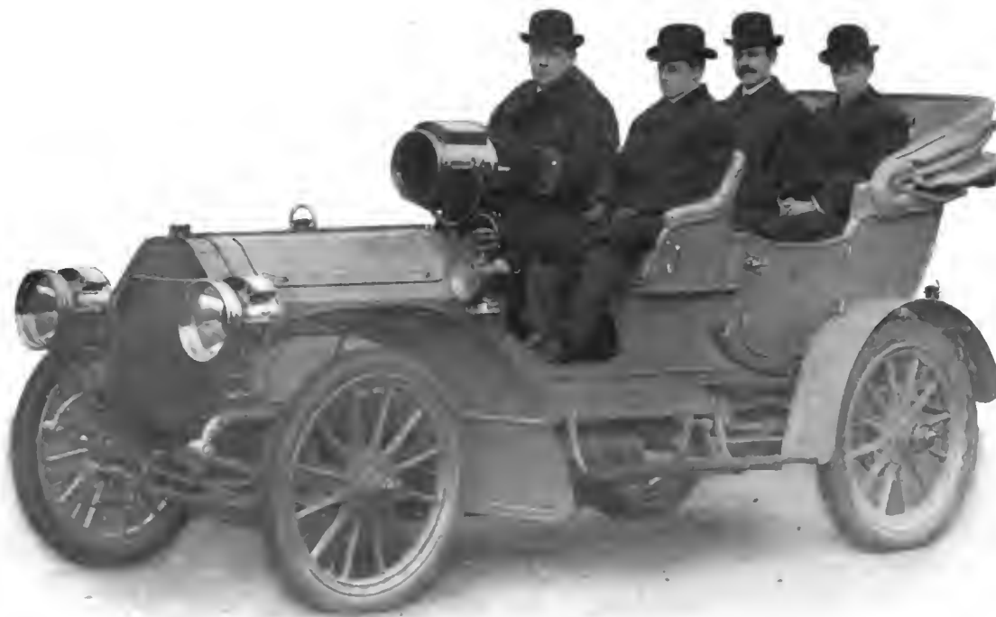
PEERLESS 1905 SIDE-ENTRANCE TOURING CAR FITTED WITH 50-H.P. MOTOR.
